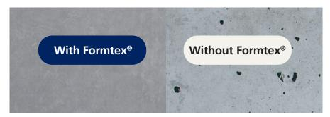
Formtex® drains surplus water and air, providing for a denser concrete cover layer without blowholes. The result is increased resistance to degradation from penetration of chloride, water, carbon dioxide and frost/thaw.
