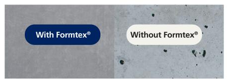
Formtex<sup>®</sup> drains surplus water and air, providing for a denser concrete cover layer without blowholes. The result is increased resistance to degradation from penetration of chloride, water, carbon dioxide and frost/thaw.
